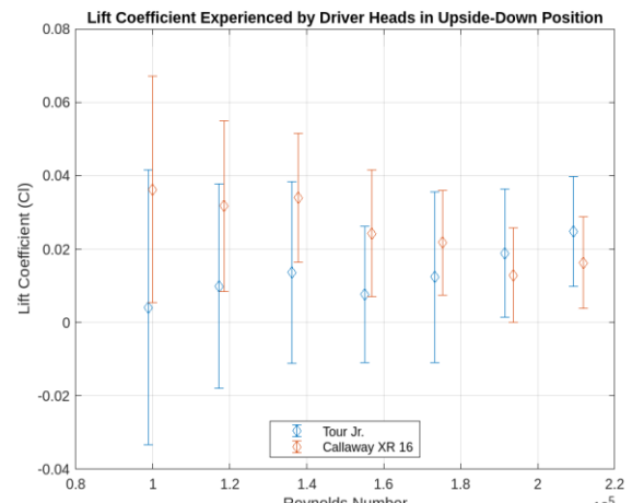
Fig. 4.2.4 Measured lift coefficient experience on both driver heads in the Upside-Down Position. Error bar is at a 95% confidence interval.
