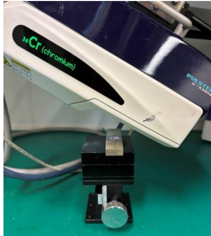
Figure 7. Pulstec micro-X360 x-ray diffraction system to measure residual stress in hybrid AM.
